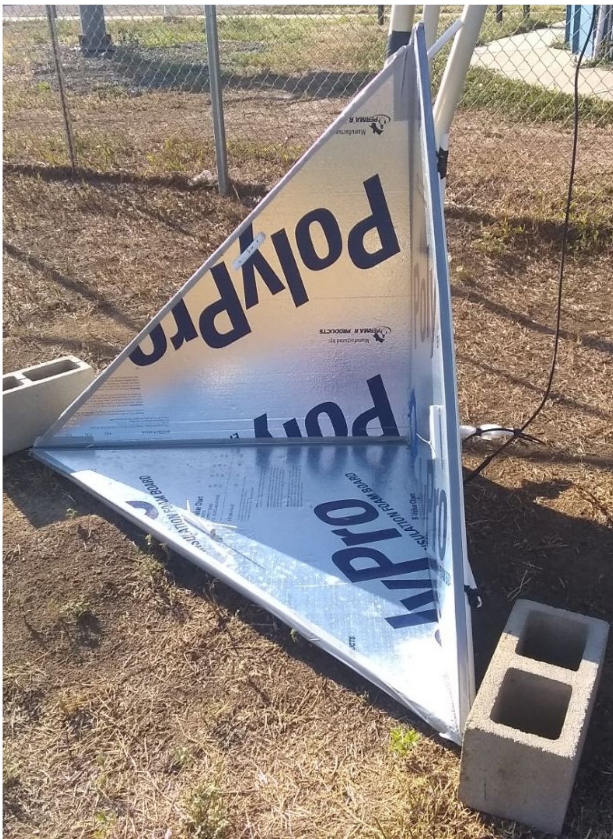
4 foot 3-Sided Corner Reflector, Berthoud Colorado USA, Little Thompson Observatory (LTO) https://www.starkids.org/visit/
