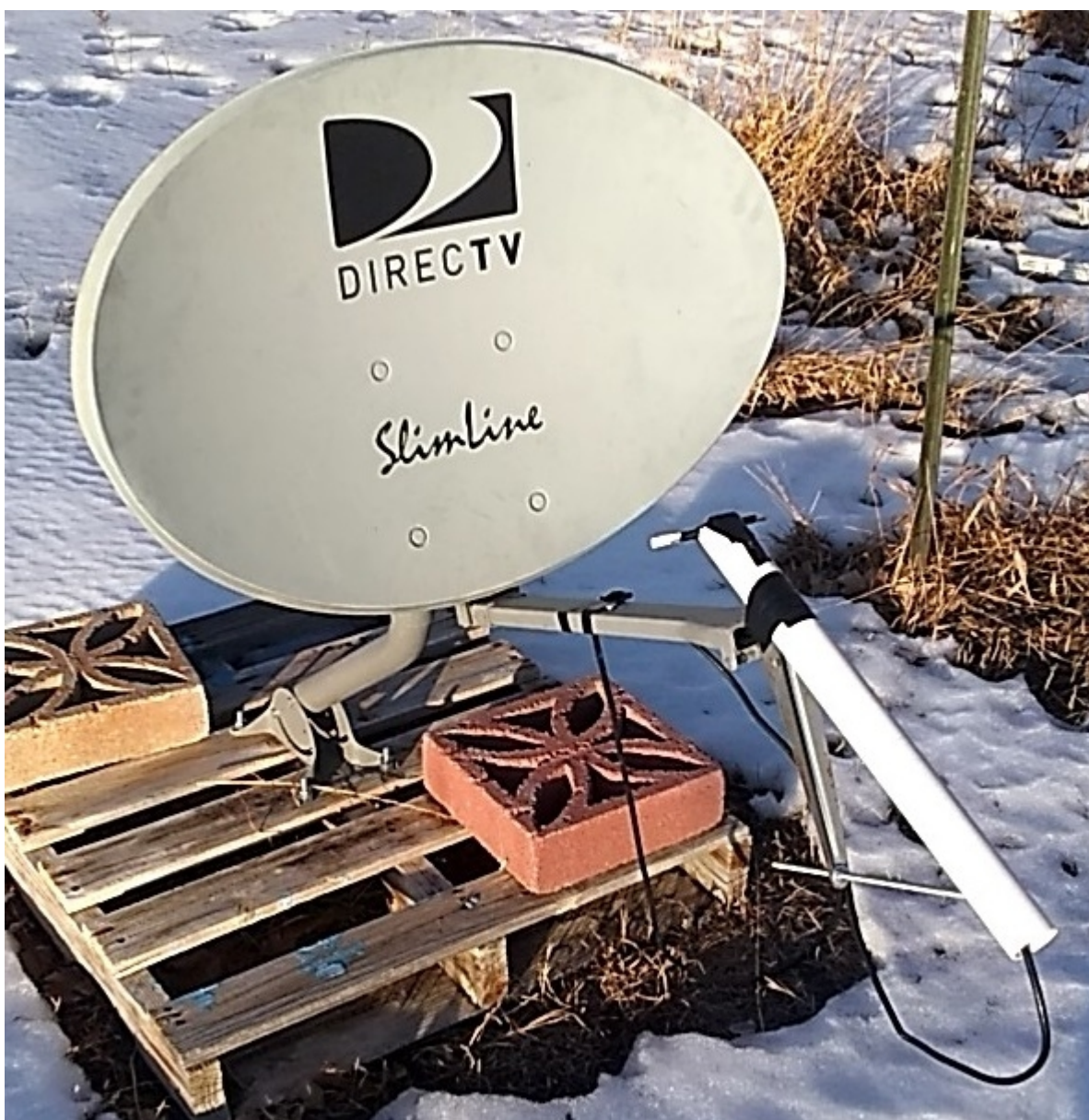
DirectTV dish with dipole, Loveland Colorado USA, N0RQV
