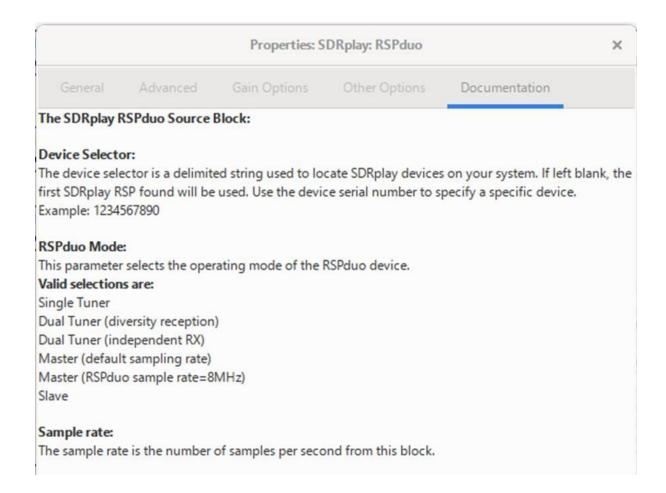
The following are the settings used in the GNU Radio SDRplay:RSPduo module to select my two RSPduo devices individually, running each as single tuner (which allows full 10MHz bandwidth to be used). Connecting the two clocks together on the two devices then allows interferometry be carried out using the two receivers at 10MHz.
