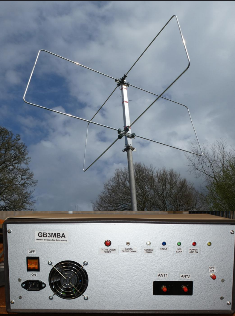
Top Left: Vertical 1m crossed Moxon Antenna - 50.408 Mhz.
