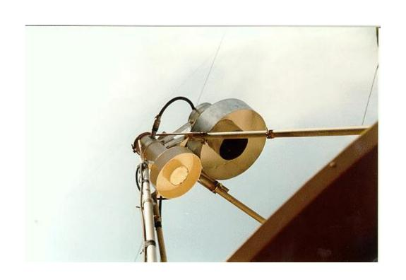
Dual feedhorns installed on EA3UM 5m SETI dish. These cylindrical waveguide feedhorns utilize choke rings of VE4MA design.
