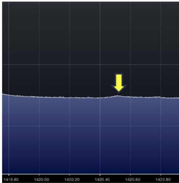
2 ) See in Real Time : Large & Small amounts of RFI and turn off the monitor or appliance before it disrupts hours of data collection !
