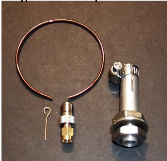
F-type <> SMA Adapter soldered to 21cm circumference wire loop
