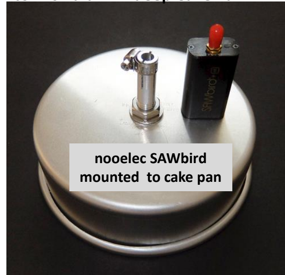
noelec SAWbird H1 SMA attached to 6" dia x 2" deep Cake Pan
